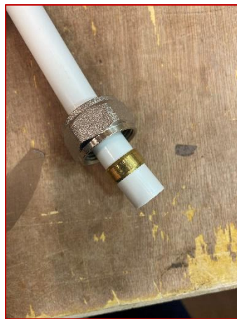
Fig. 8.2 - Pipe with Eurocone nut and compression olive.
