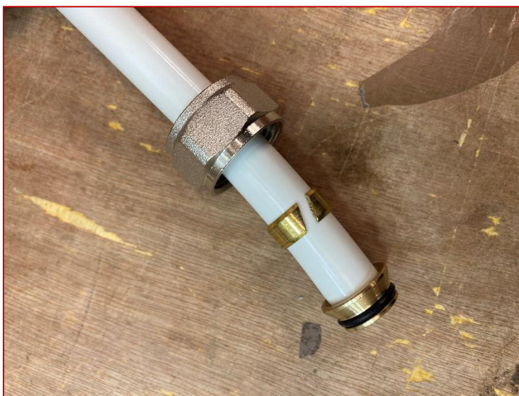
Fig. 8.3 - Pipe with Eurocone nut, compression olive and push fitting inserted.
