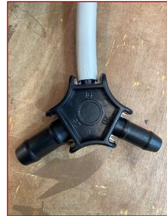
Fig. 7.2- Reaming tool with the correctly sized node inserted into the pipe.
